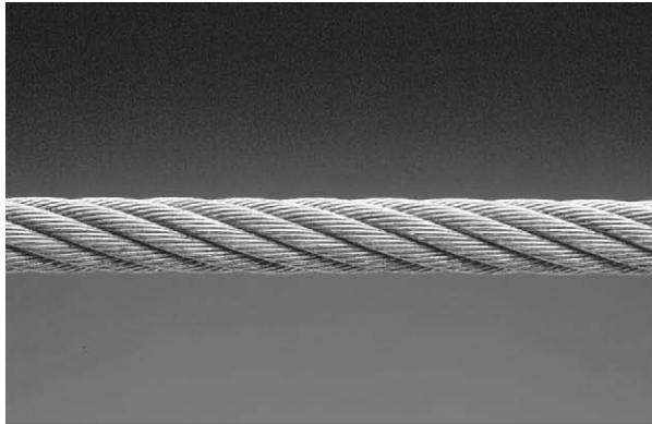
Typical Good Cable
