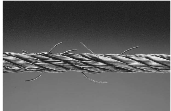
Cable With Broken Wires
